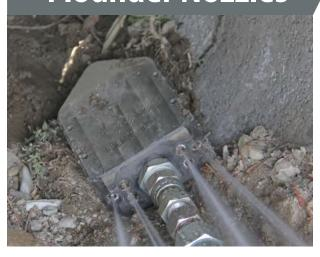
In the sewerage networks with a rather large diameter and many sands cluttered and settled in layers at the bottom of the channel and water flows in the channel, where the only access for clearance is from the opposite direction of the water flow, submarine Flounder nozzle is simply placed at the bottom of the channel among the sands.
