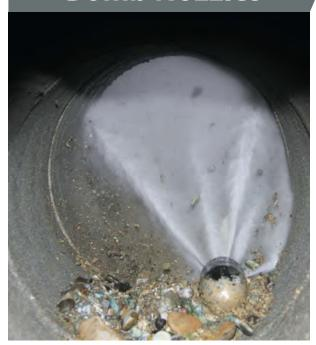
This nozzle is made of hardened stainless steel; due to the heavy weight and backward outlet jet patterns which are in two different angles (10° & 30°), the nozzle has great power and can easily pass through the pipes by hitting the materials inside the pipes.
