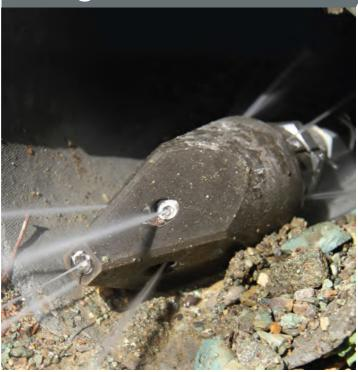
When the sewerage pipe is thoroughly blocked, the best device to remove the blockage is SMC Angle-faced nozzle.
