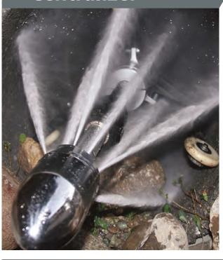
Centralizer is one of the equipment used for nozzle movement in the center of sewer pipes. Umbrella mechanism has been used in design of the centralizer to increase adjustment speed. To reduce the weight and prevent from the sparkles in the pipes due to the flammable gases, the equipment is made of Aluminum with a special anti-sparkle cover.
